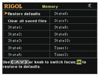
It supports storing and recalling state files and timer files, and allows you to restore the instrument settings to defaults
